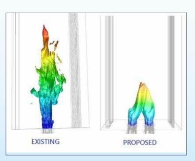
Existing burner configuration has longer and wider high temperature zone. Proposed smaller burners had shorter high temperature zone.
