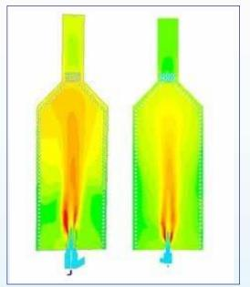
Comparison of flame profiles and path lines show that proposed case flames are shorter and better flue gas circulation pattern in the heater to reduce radiant tube metal temperatures.
