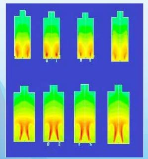
Temperature contours on various angular planes in the heater were compared for the existing and inclined firing case. Inclined firing clearly shows the flue gas temperatures around the radiant tubes is reduced which helped in increasing the run time of the heater.
