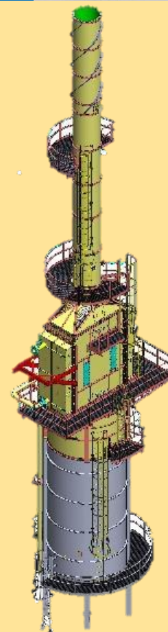
DHT Charge Heater (210-H-100) Capacity Improvement
